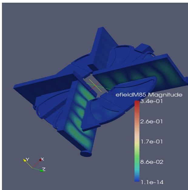
Figure 1: Electromagnetic simulations of the full PSI Ring Cyclotron vacuum volume with old aluminium cavities but without the flat-top cavity.
